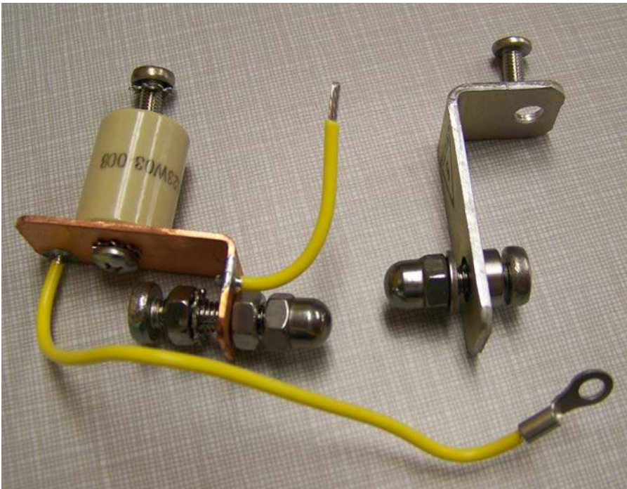
Figure 5: Spark Gap Assembly 197-8067-01 (showing HV16 terminal lug), for use with NAFP07
