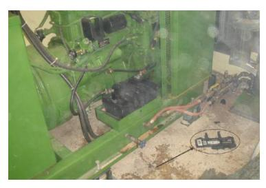
Baun was happy to report that no one was injured when this battery failed. (You can see the top was blown off and is laying on the ground in pieces – the cells are exposed.)
