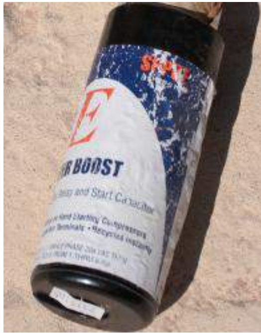
An air conditioning unit capacitor
