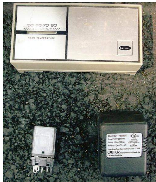
A low voltage gear thermostat, relay, and 12 VDC transformer
