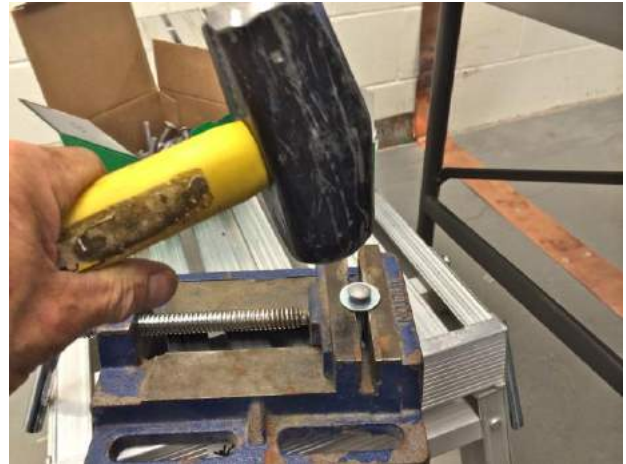
Adapting ¼ inch x 20 carriage bolts to accept ¼ inch fender washers
