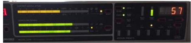
Showing the 57 kHz RDS modulation using a 2-foot wire antenna
