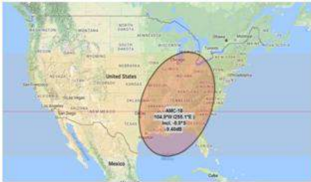
Illustration 1: Sun Outage Foot Print from www.satellite-calculations.com showing the approximate area of sun outage for SES-11 at 13:20cdt 03/06/2018. The site will even calculate the approximate amount of C/N loss during the sun's transit based on entered system specs. Here it is -9.40dB.
