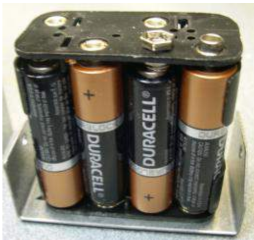
Eight AA batteries are used in the BE675A
