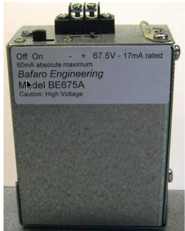
The BE675A. Note the on/off switch on the left side, to enhance the battery life.
