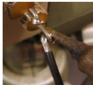
Here is the most important point in the whole process! The solder flows *toward* the heat source, and this dictates where you place the iron and introduce the solder.
