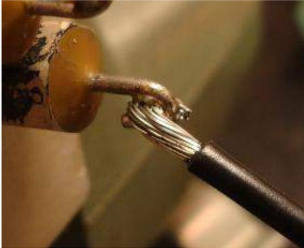
**A good joint does not need globs of solder**
