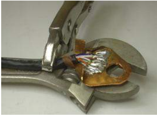
CAT5 cable was soldered to a piece of copper strap
