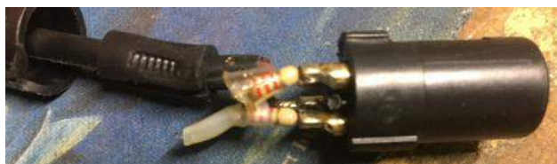
Placing the 2.2k resistors in the XLR input
