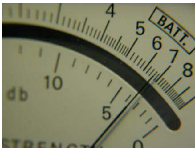
Typical reading with a new pack of AA batteries
