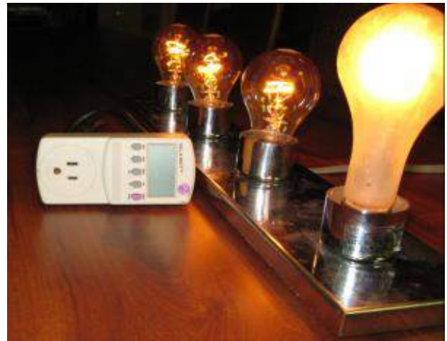
With the lamps on line, the full capacity of a UPS can be tested
