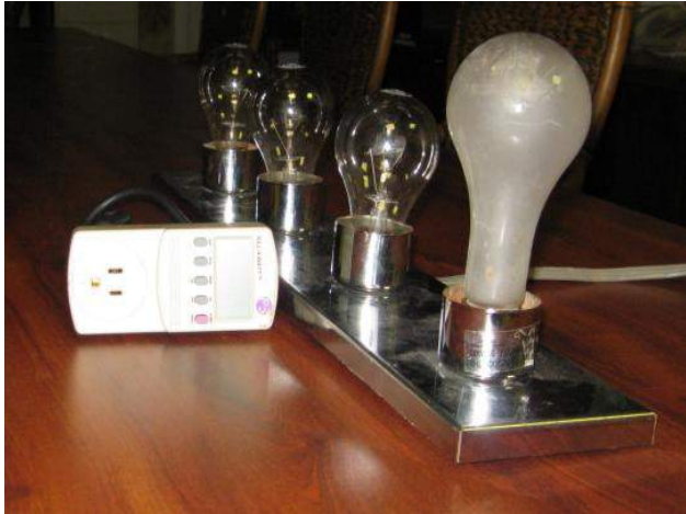
One 150-Watt and three 116-Watt lamps were used to provide a load of up to about 500 Watts
