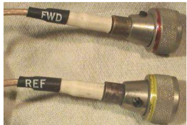
VSWR sample lines. Notice the color banding
