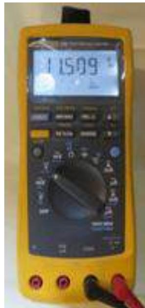
The Fluke 189 was available by 2000. It is a true RMS 5-digit logging DMM with the normal ranges plus capacitance. Using accessories it can be connected to a computer to download the log-ged information. I do not believe that it is still available, but all of its functionality (and more) is available in current 287/289 meters, although it is north of \$500.
