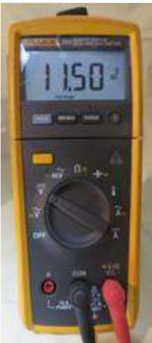
This looks a lot like a normal Fluke DMM, but the display section can be pulled off, and will continue to read up to 30 feet’ or so from the rest of the meter.
