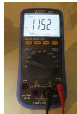
The B35T measures Volts up to 1000 V, with a .1 mV resolution up to 60 V, Amps, frequency, and temperature.
