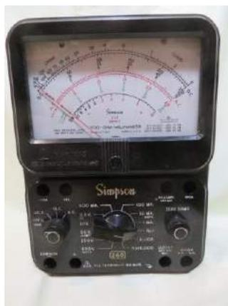
According to the a00201939 manual, “The Model 260 Test Unit offers the serviceman a small, compact and complete instrument with high sensitivity for testing and locating trouble in all types of circuits.”
