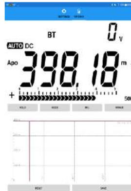
This meter has features like low burden Voltage in current measurements. The software is open source. One slightly unusual feature is an internal ambient temperature measurement.
