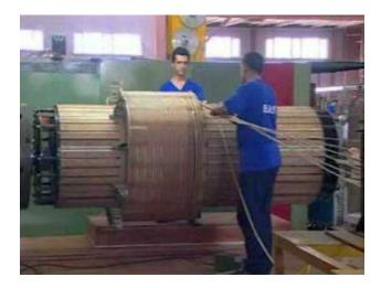
Two coil winders engaged in the painstaking task of fabricating the heart of a transformer. The right end of the cylinder is supported by a free-running bearing. The left end of the cylinder is supported by a motorized mandrel. See the <u>full video here</u>.
