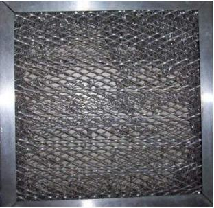
As you can see, the metal filter has deteriorated and internal pieces are breaking off.
