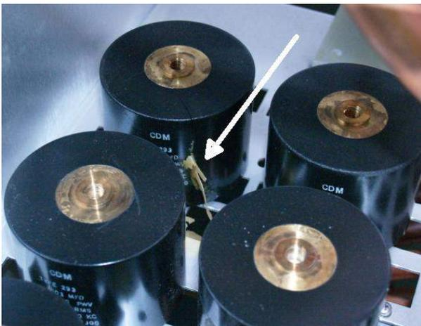
**The wax escaping from this capacitor is a good sign that it is an ex-capacitor**
