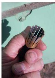
Since similar tube sockets I had previously stumbled on were already damaged I have to admit I have never actually watched a filament connection corrode.
