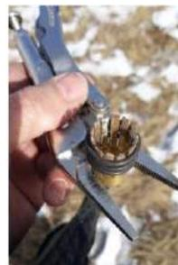
Cleaning up the surface of the socket and then reinstalling it brought everything back to normal.
