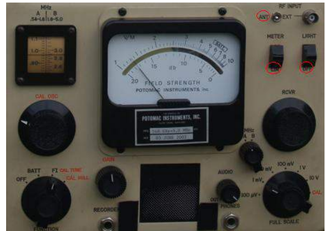
Set the Meter for the internal antenna, LIN mode, and light off
