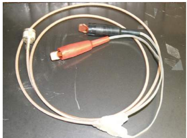
Some sturdy homemade test leads
