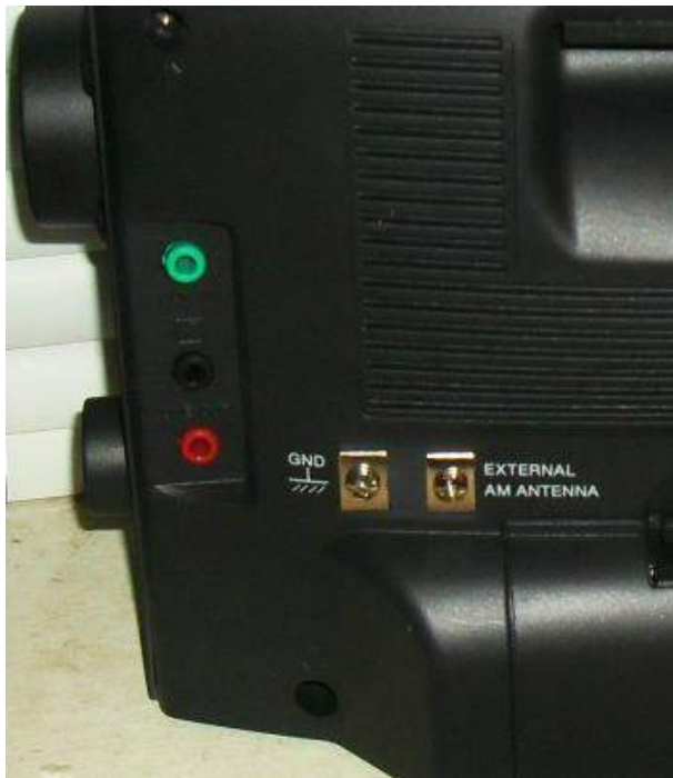
The rear of the radio has AM antenna screws, Aux In (green jack), Line Out (red), and a timer switch (black). The battery compartment holds 4 D Cells.
