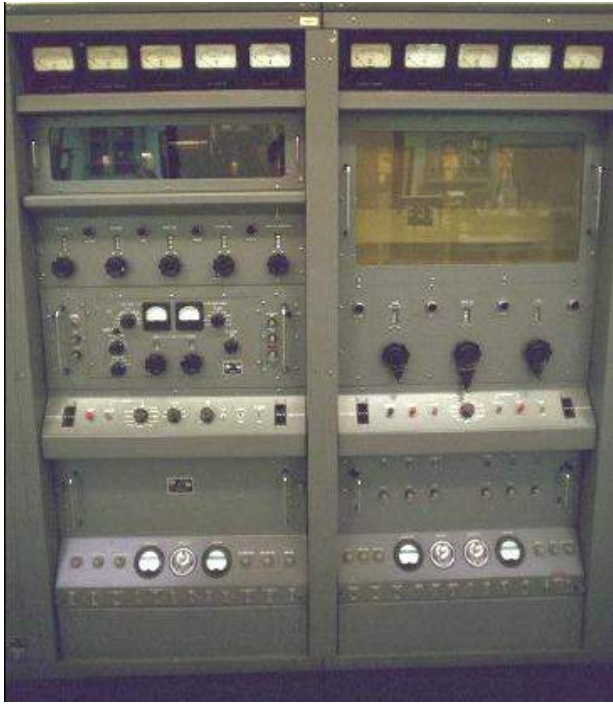
NIST picture of part of WWV's 5 MHz transmitter
