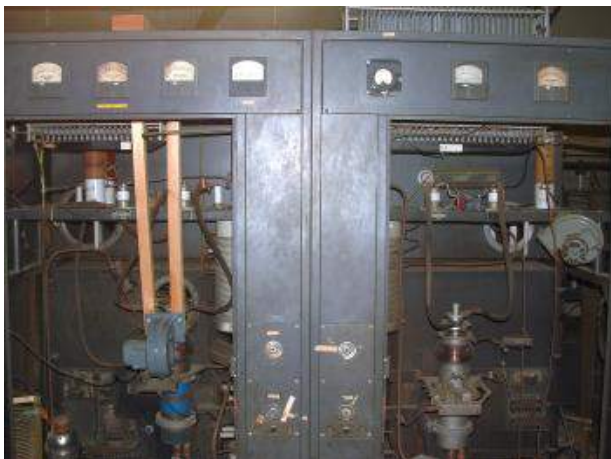
The 407-A4 Carrier and Peak tubes
