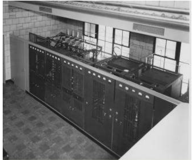
The WE 407-A from above – notice the open back
