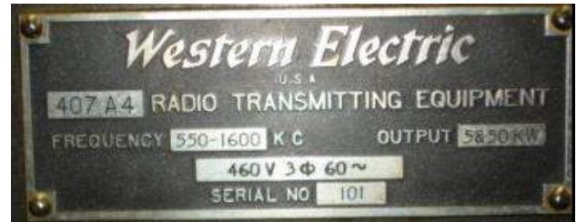
The nameplate from the WTOP transmitter “Output 5850 kW”
