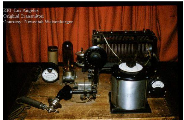
Earl C. Anthony's first transmitter was a true "breadboard" construction.
