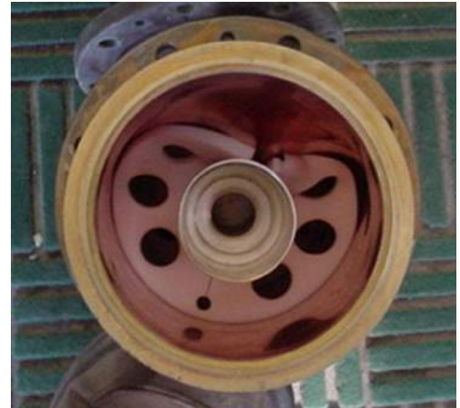
This elbow was damaged when a crew working for a co-located station dropped a 10-foot piece of conduit on it – and was then ready to leave the site without telling anyone. Photos: Gary Peterson
