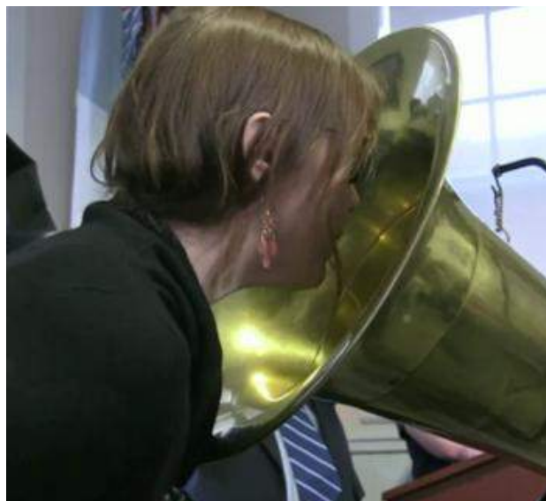
The horn was microphone and speaker
