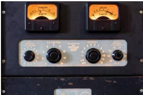
The PROGAR brought automatic gain control and peaking limiting together.
