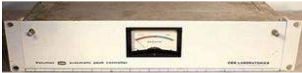
The Volumax provided a limiter to complement the Audimax
