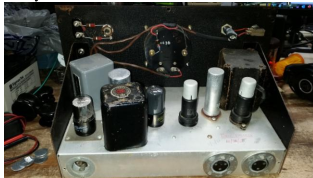
Rear view showing AC power socket, microphone inputs, tubes, transformers, etc.
