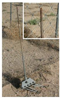
On the left, you can see the guy anchor that failed, with a close-up of the point of failure in the inset.
