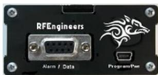
The only other connections, on the back, are a smaller USB Type B jack like you find on smart phones, and a DB9 jack.
