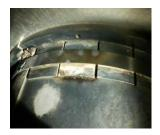
Hartman also provided this photo of a tube plate blocker that was seated improperly by someone inexperienced with this type of transmitter.
