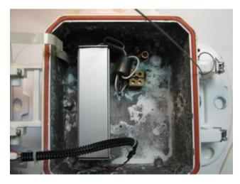
After we dried it out and, as a test, temporarily bypassed the power connection strip which was severely corroded, the light came on immediately with no indication of any malfunction.
