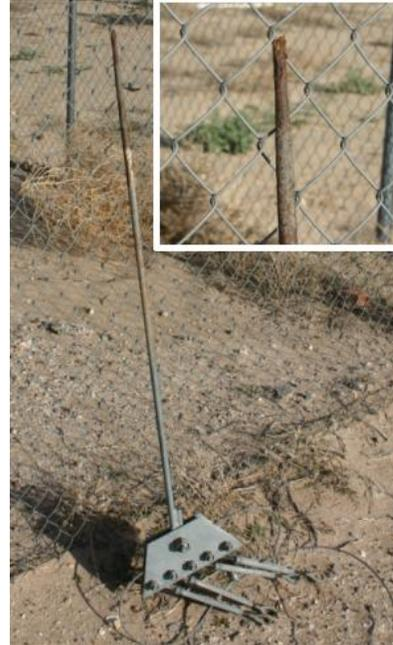
On the left, you can see the guy anchor that failed, with a close-up of the point of failure in the inset.
