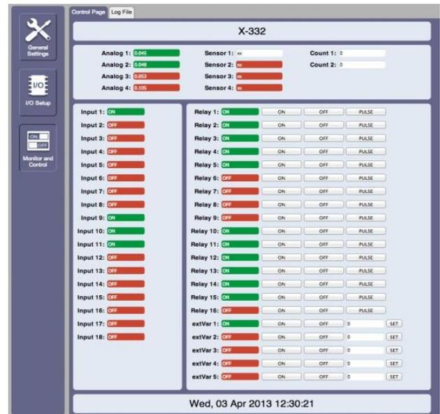
It has 16 digital inputs, 4 analog inputs, and 4 separate temp sensor inputs. It also provides 16 relay controls that will either pulse or latch.
