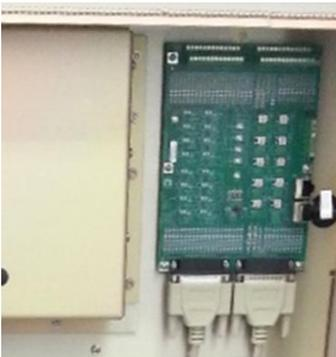
The controller also has another trick to it: the “mimic panel” where all your local wiring goes as well as an Ethernet pass-through jack for remote control. It has the basic control buttons on it
