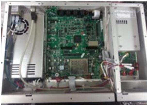
There is a main board with the RF generation section, an audio section, and a little RF out going into a PA brick on the right side in a walled-off cavity for RFI suppression.
