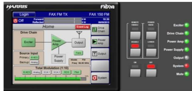
Although it does not give you a pretty spectrum analyzer for the RF or a constellation of the audio, it does give you plenty of metering from audio to the RF stages, including temperature sensors pretty much at every point from AC in to RF out, to control any over-temp situation.
