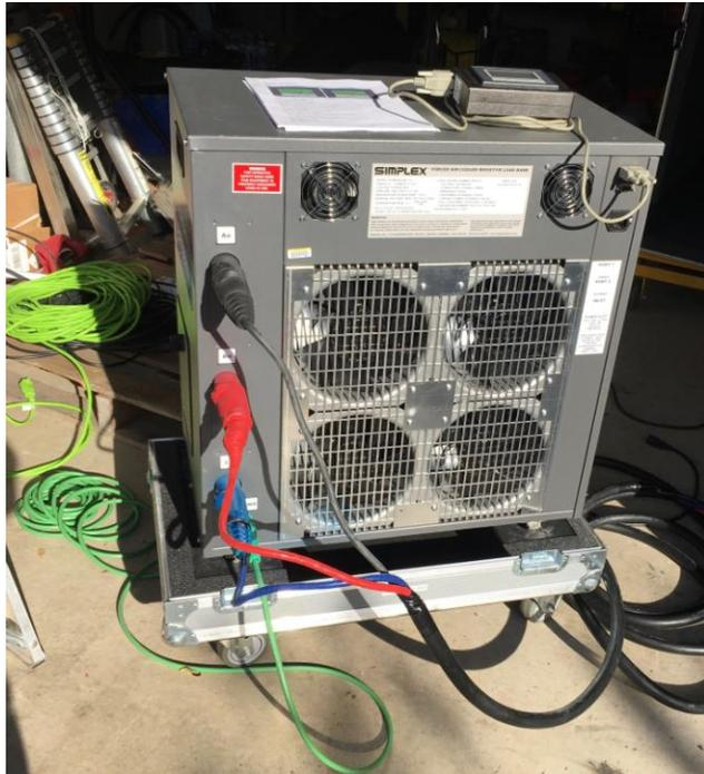
**110 kW simplex load bank with 3-phase, neutral and ground cables**
