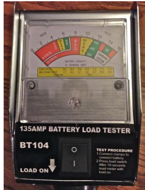
This battery load tester will draw a lot of Amps
