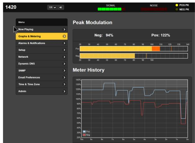
As part of the clear and comprehensive series of menu options, the unit has an easy to use email area for up to 10 different addresses and each address can be programmed individually as to what notifications each one should receive. As SNMP is becoming more popular for facility monitoring, a configurable interface is also included for stations that want to use it.
