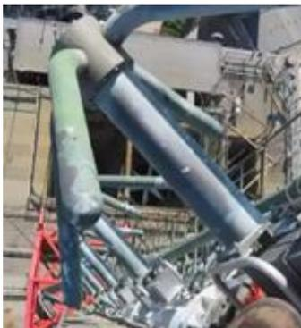
The antenna had an internal pressurized feed enclosed in a fiberglass insulator. The insulators in the antenna elements had deteriorated from exposure to the sun.
