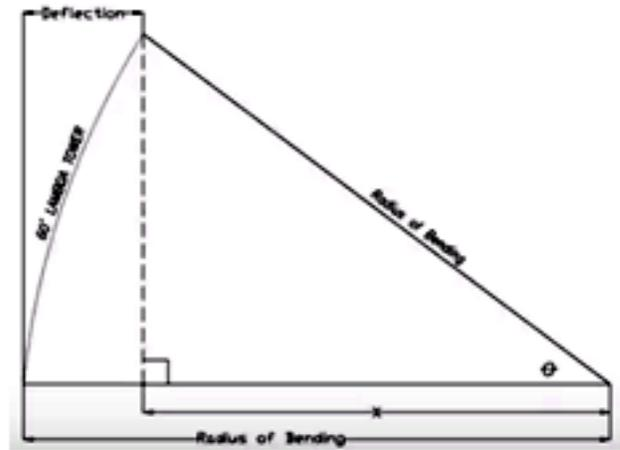
You can see in the example above that the tower forms an arc and the radius of bending is the same at the top as it is at the bottom. I published a paper on this years ago because everybody kept asking how you calculate uniform tower deflection.
