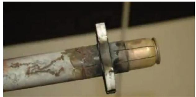
This is what the bullet looked like. We replaced the bullet, cleaned up the outer conductor, placed the inner conductor back, put it all back together – and the noise problem stopped.
