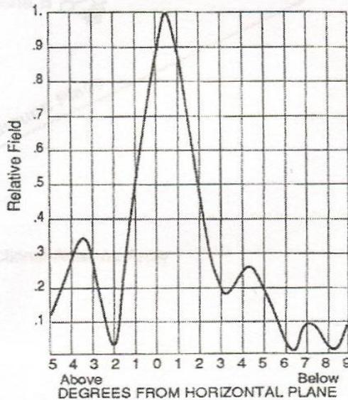
Figure 2 - Effective Field of a Vertically Stacked Antenna
