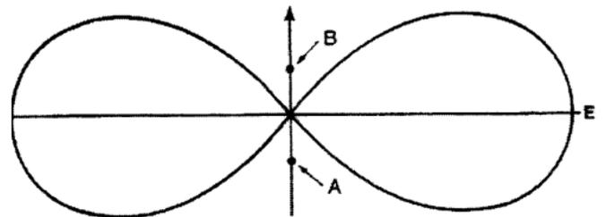
Figure 4 - The Effective Field of a Two-Element Array
