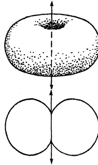
Figure 7 - Field from a single vertically polarized FM antenna. The arrows represent the antenna axis, or direction of the dipole element
