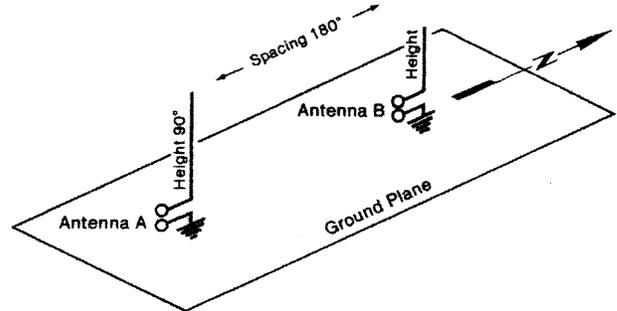
Figure 3 – A Two-Element AM Directional Array
