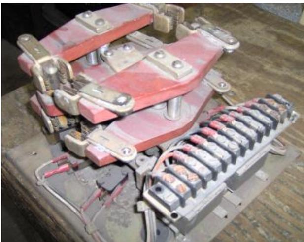
**The contactor was submerged in water in a flood**
