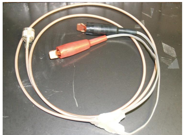
Some sturdy homemade test leads
