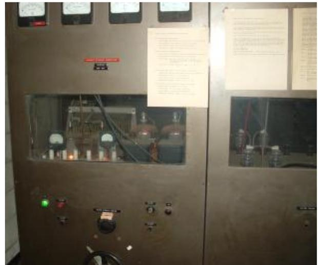
**The original, homemade 1 kW WFLI transmitter**
