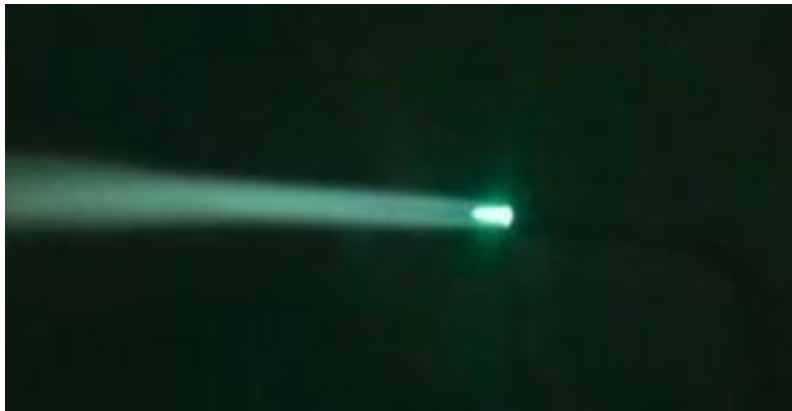
The tip of the inner cone is hottest point.
