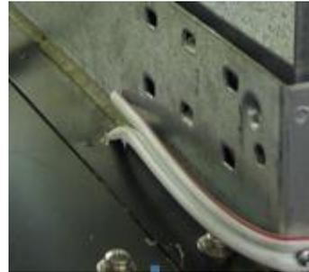
14. From the top of the transmitter, drill a hole in the back corner of the fan housing, below the lip that used to hold the steel rod or expanded mesh assembly that supported the foam filter.
