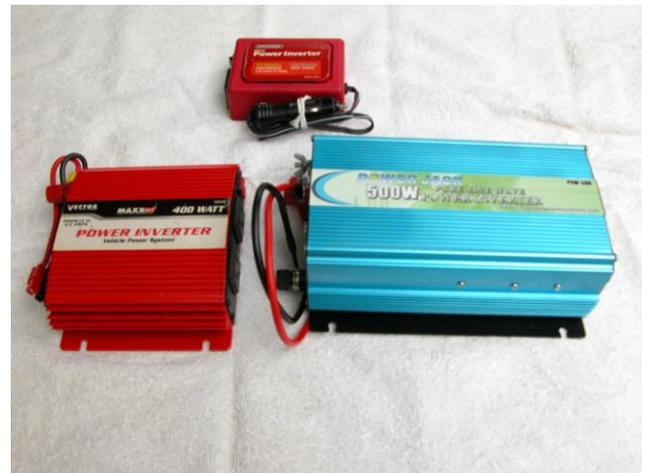
**Top:** Ray-O-Vac, 75 Watts, modified sine-wave
