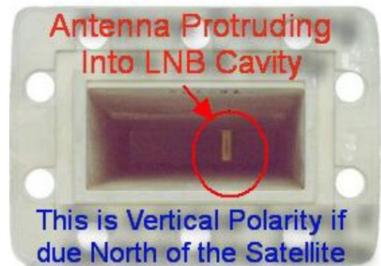
Turn it until it points straight up or down and that is vertical. Then rotate the LNB to the preliminary location per the skew instructions. The wide dimension of the LNB will be laying horizontal(ish) when the little antenna is vertical.
