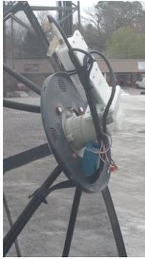
These servo movable “hair-pin” type feeds have at least 10 dB (and some have over 30 dB) less cross-polarity rejection than a standard professional type LNB mount. Since smaller and mesh dishes struggle to meet 2° satellite spacing, be aware that you can improve
