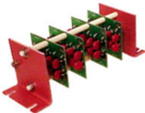
For example, this stack or composite of components is very complex to test. The device pictured consists of twenty type 1N3495 diodes.
