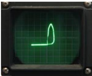
Close observation of the curve trace shows a variation from the normal straight-edged perpendicular trace.
